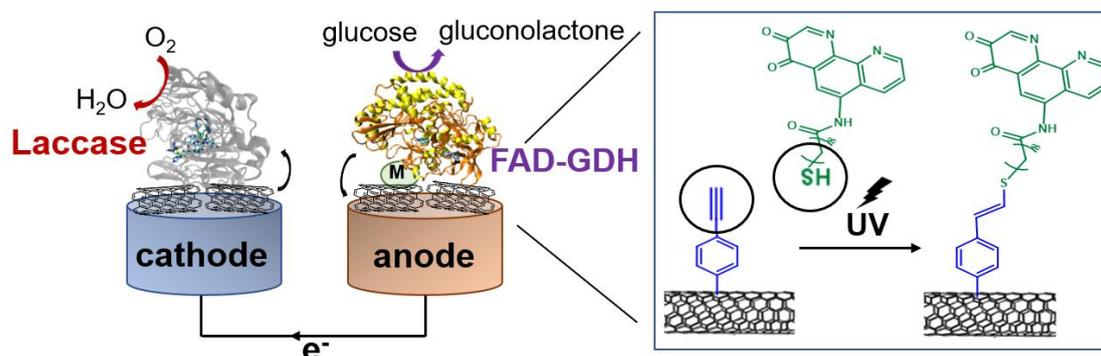
**Figure 1: Scheme of an enzymatic biofuel cell constituted by laccase enzyme at the cathode and FAD-GDH enzyme at the anode after immobilization of thiol redox mediators onto alkyne modified carbon nanotubes by thiol-yne chemistry.**
