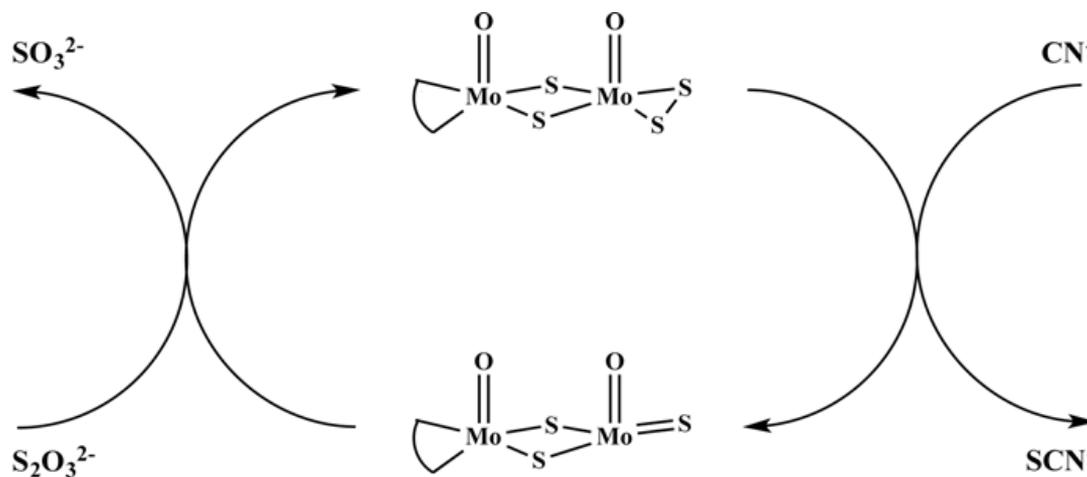
Figure 1: Catalytic cycle of molybdenum complex and cyanide<sup>2</sup>
